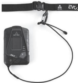
Position the EVO5 in a zippered pant pocket for the entire duration of your outing. The zipper slider should be fully closed, leaving only enough room for the elastic cord to exit. Adjust the belt around your waist and then buckle it.
