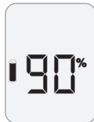
The device then displays the software version installed and remaining battery life. We recommend that you replace the battery as soon as it drops below 50%. Holding down the marking button in transmit mode will allow you to check battery life left at any time.
