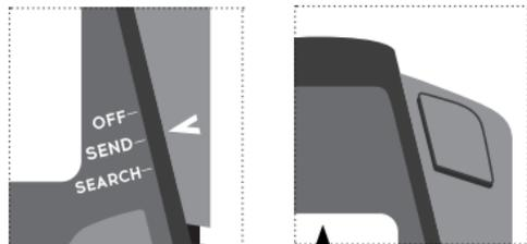
The selector is properly locked when, in transmit mode, the lock button pops out and you hear it click into place and you cannot push it down any further.
