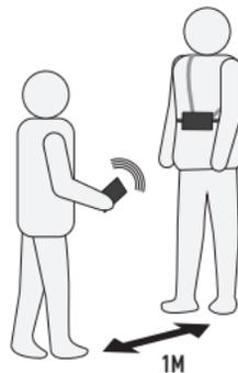
In GROUP CHECK mode, the EV05 starts by analyzing the transmit frequency. If the frequency does not comply with current standards, a "no" message will appear indicating that the device being checked is defective and should be sent to customer service. If the frequency meets the standard, a distance reading will display on your screen and you may then proceed to checking transmit power :
